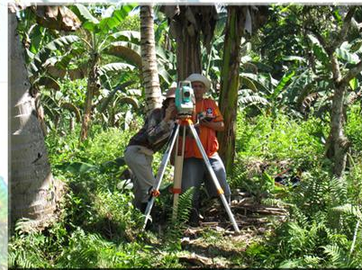
PHIVOLCS personnel use Total Station surveying instrument to map active faults in the field
